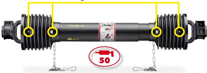
The standard lubrication frequency for all components of series Global cardan joint drivelines is 50 hours. This lengthens the lubrication interval from a daily chore to a weekly routine. Grease fittings are aligned and easy to access.
